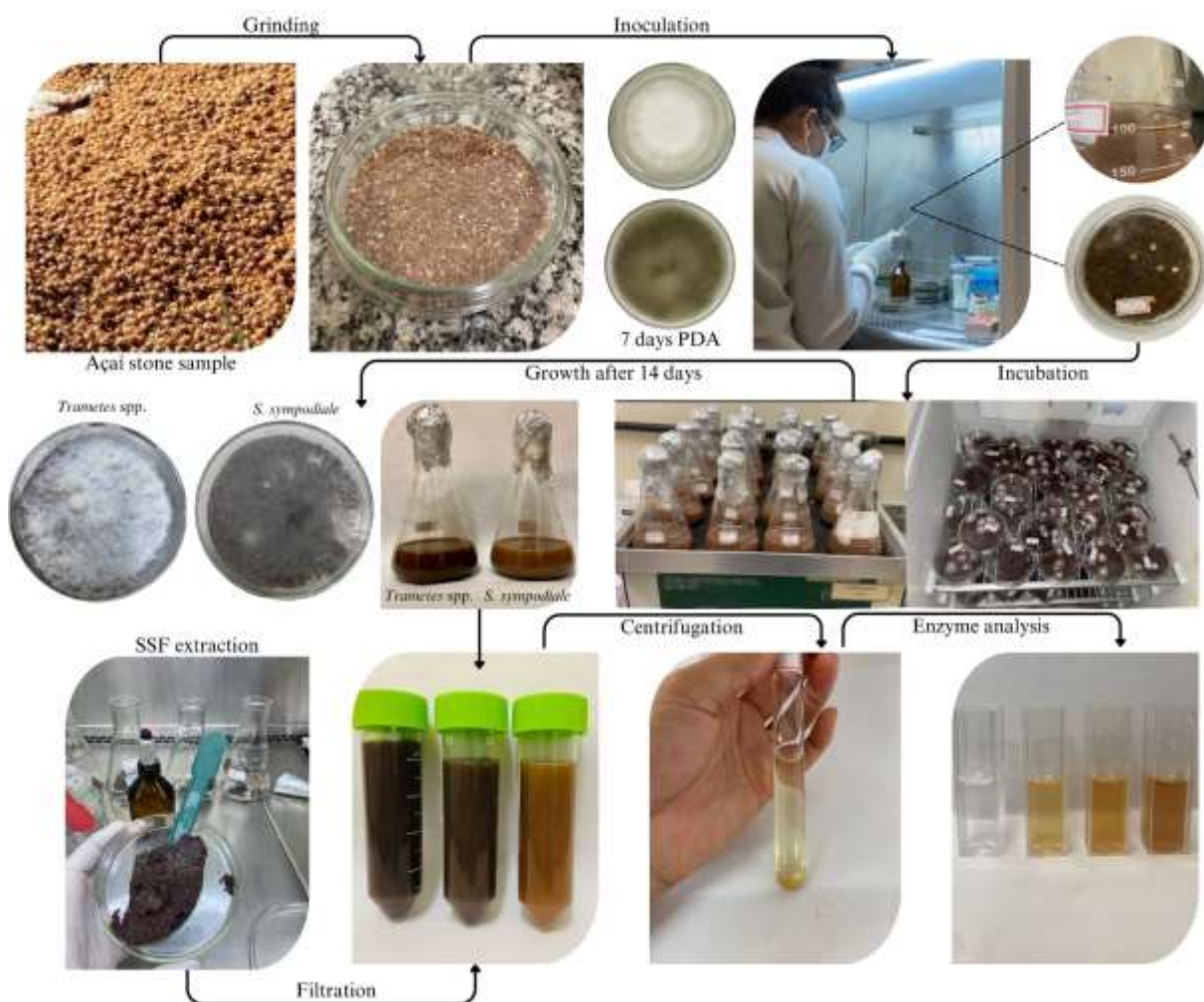
Figure 1. Schematic process of solid-state fermentation (SSF) and submerged fermentation (SmF) of the açai seed and extraction of the enzymatic substrate.
